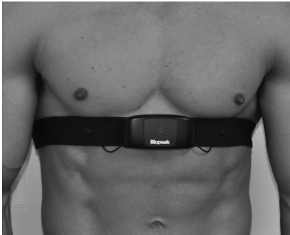
Fig. 1. Biopeak chest belt system acquiring data from healthy male subject. It comprises two active rigid electrodes on inner surface of belt (not seen). These electrodes are connected to central unit, which attaches to outer surface of belt as shown.
